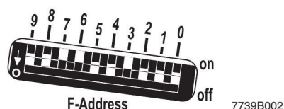
Figure 2-9 Switch for F_Destination_Address (F_Dest_Add)
